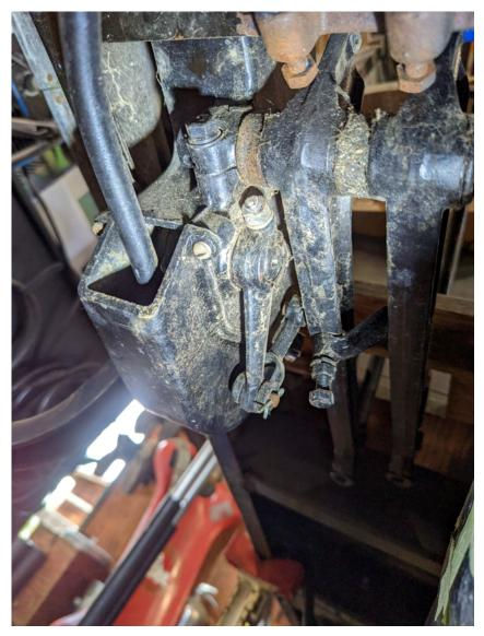
During the restoration of my 1917 Detroit Electric model 68, I removed the parking brake ratchet box from the chassis for cleaning and refinishing.
