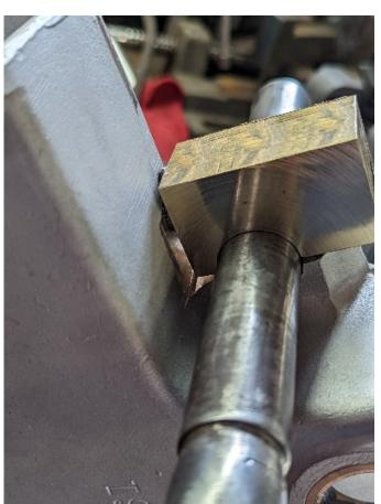
The next step was to drill the hole for the clamp bolt. I made a pointed piece of a bolt to install in the mounting hole; a tap with a hammer marked the position to drill the hole in the clamp.
