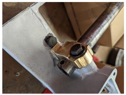
It works! A little filing of the clamp tang and the fix is complete. It holds the pedal shaft firmly and is much stronger than the original design. Now the box and parts can get painted and reassembled.
