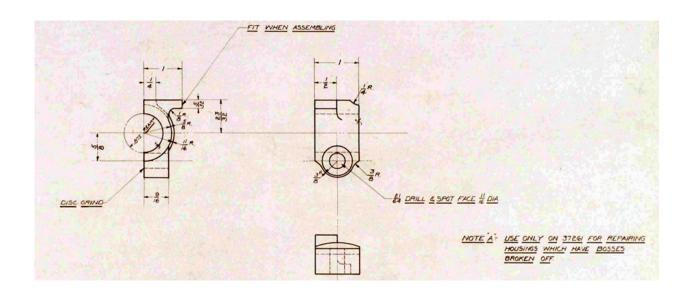
My shop has a miscellaneous collection of tools, but is far from a full machine shop; I had to do this with what I have. I started by machining off the broken bracket. I used my woodworking radial arm saw, fitted with a "non-ferrous metal" carbide blade, slicing off the parts as indicated in the drawing.
