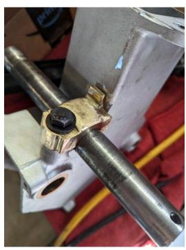
The last step is to place the support bolt in the housing. The drawing is not complete in the dimension of the placement of the bolt, but since I left the clamp tang long, the placement of the bolt is not highly critical. I drilled the hole and added the bolt and nut.
