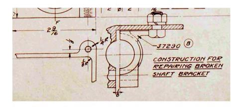
It seems that the company had experience with this part breaking and identified it as a design flaw. They designed a fix which includes removing part of the existing clamp that is prone to breakage, installing a support bolt, and they designed a replacement part that implements the missing part of the clamp. Another search of the Electric Vehicle Archive and I found the drawing for the replacement part. The solution is now in hand, I just had to implement it.
